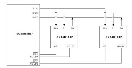
Figure 3. System Configuration Using SPI nvSRAM
